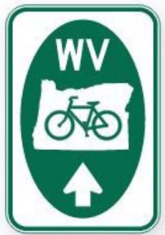
Bicycle route guide signs are used to indicate a preferred route for bicyclists. They should be used when the signed route provides a clear advantage to bicyclists such as: a low volume street, a short cut, a flatter route, a bicycle boulevard, a bicycle specific destination, or an alternate to a busy, bicycle unfriendly thoroughfare.
